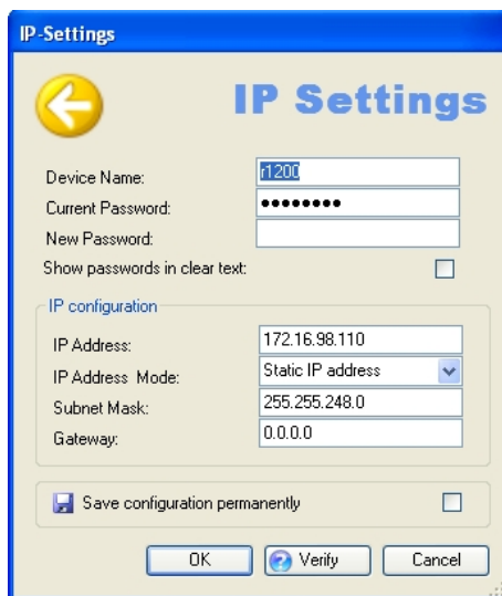
Fig. 4: IP address allocation using Dime Manager
